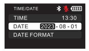
DATE FORMAT can be set, and in the "DATE/TIME" setting, you can see a variety of date formats to choose from. You can choose a common date format: "DD/MM/YY", "MM/DD/YY" or "YY/MM/DD". You can select the corresponding date/time format by pressing the up and down keys and click OK to save the selected settings. The date and time format shall not be saved by clicking Back.
