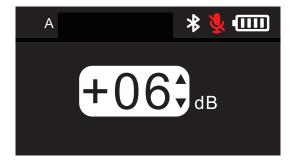
Long press the "Down direction key" to enter the output gain adjustment mode of the output port B. You can adjust the output gain through the "Up/Down" direction key. There are 31 gears of gain adjustment, and the gain can be customized according to the usage scene. The adjustable output range is -20  $\sim$  +10dB.
