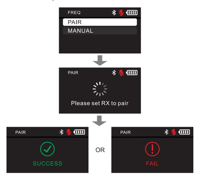
**Networking mode II of DBTX and D2RX:** it is needed to manually set DBTX and D2RX to the same frequency point to complete the pairing networking.
