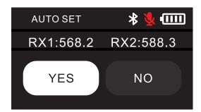
Click "YES" to send the synchronously scanned frequency points to the transmitter, and click "NO" to cancel the synchronous frequency point distribution.
