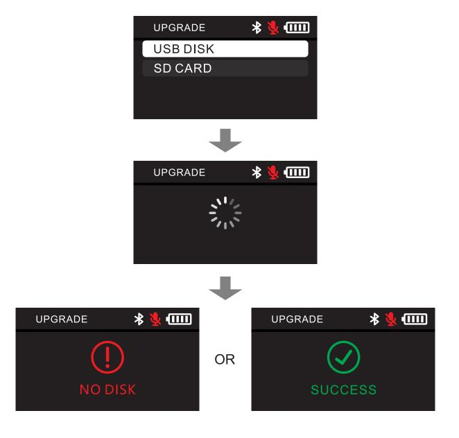
Insert the SD card into the device, select the "UPGRADE" option in the menu, and update the firmware according to the screen prompts. After the firmware update is completed, the device will automatically restart, and the firmware version will display the latest version number. You can enter the "Firmware" option in the system settings menu to inquire about the firmware version information of the current device.
