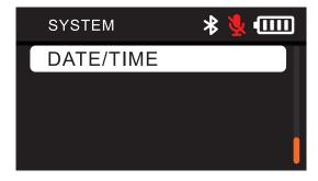
You can customize the current time information for the device. Click OK to enter the time adjustment. Press the up and down keys to adjust the time number. After the adjustment is completed, click OK to save the set time information, and click Back to return to the time information set last time or initially.
