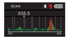
The optimal frequency point can be automatically distributed after the frequency scanning
