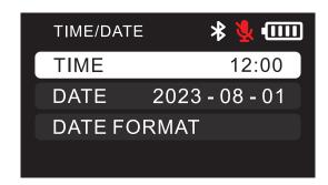
DATE setting can customize the current date information for the device. Click OK to enter the date adjustment. Press the up and down keys to adjust the date number. After the adjustment is completed, click OK to save the set date information, and click Back to return to the date information set last time or initially.
