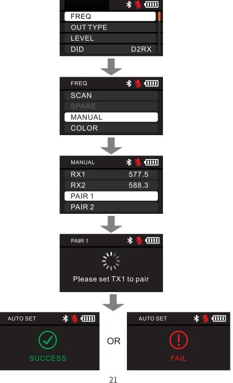
**DBTX:** Select "FREQ" mode through the menu in DBTX, and then enter the pairing mode by selecting PAIR with the up and down keys, and "SUCCESS" will be displayed if the pairing is successful. If the pairing fails, "FAIL" will be displayed. If the pairing fails, it is needed to re-pair or check whether the antenna is installed correctly.
