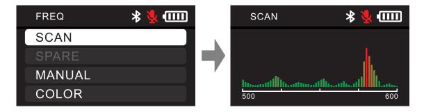
If you don't use the automatically allocated frequency point information, you can click the back key, and manually select the frequency point by "Up and Down keys" to send synchronization to TX for use according to the result of frequency scanning
