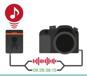
**Please note:** The built-in microphone can only be used, when working at mic levels with plugin power switched on at the camera side.
