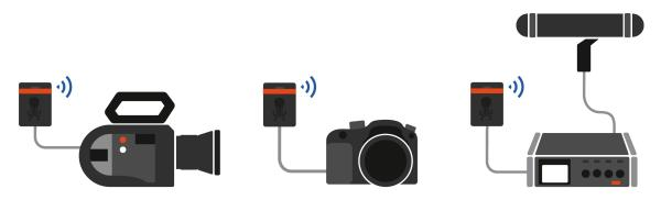
Tentacles can be used with nearly any recording device: Cameras, audio recorders, externally recording video monitors and more. All they need in order to work with a Tentacle is either a dedicated timecode input or at least one audio channel to record Audio TC on. There are basically two groups of recording equipment:
